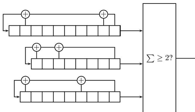
Figure 1: A simple LFSR based cryptosystem.
